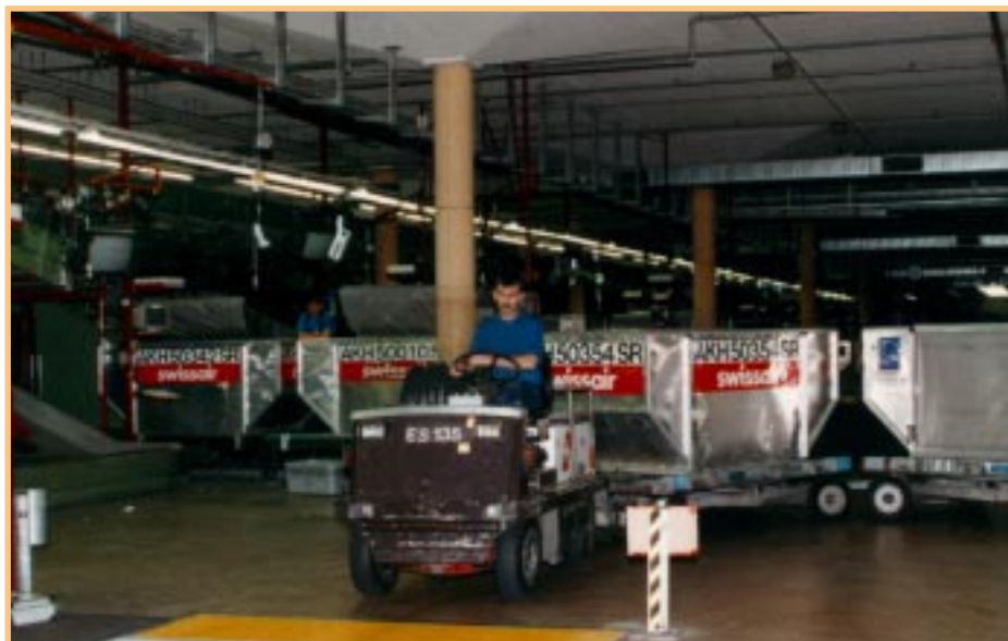
With Swiss Air's new drive-on scale, luggage wagons are weighed automatically saving time and eliminating errors.
